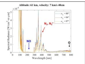
**Fig. 1**. Synthetic OES spectra predicted by NEQAIR and based on US3D simulations at different three viewing angles. Altitude = 61 km, speed = 7 km/s.
